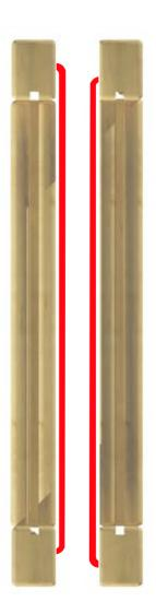
When viewing an upright, shelf support holes are offset to the left of centre on each upright pole.
